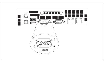
Figure 3-4. Serial Connector Location and Pinout
